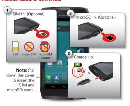
**Note:** Installing a SIM card is optional. A SIM card may be needed for roaming outside of the United States, and can be purchased from foreign carriers. To avoid SIM card damage, turn off your phone before you insert or remove the SIM card.
